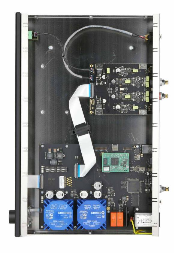
High-quality, discretely organized analog outputs, two 32-bit converter chips per channel and a powerful DSP from Analog Devices as well as a high-quality power supply form part of this high-end kit. The housing chassis is made of stainless steel.
